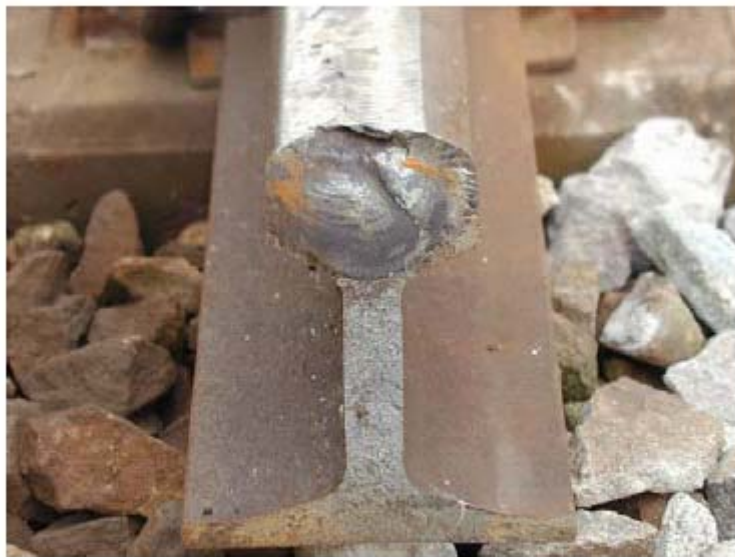
Figure 4.1 – Rail fracture at Hatfield.
